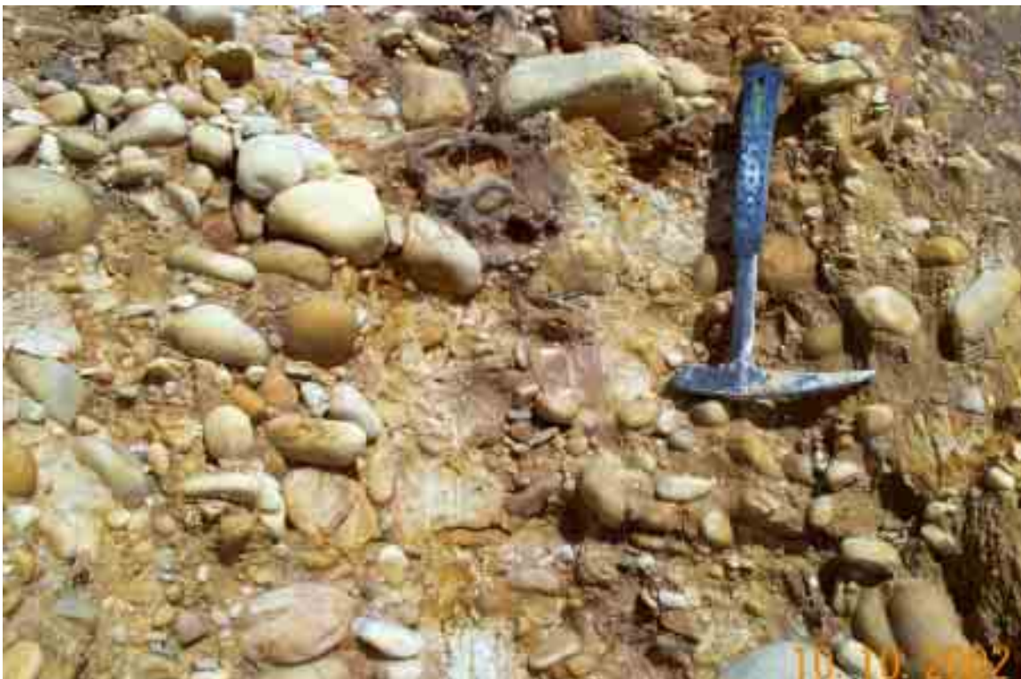
Figure 6: Detail view of silty-clay pebble/cobble alluvium at Site 40, showing hard unweathered quartzite cobbles, and soft, deeply weathered mudstone and siltstone clasts (eg, "ghost" clast outline visible immediately to LHS of hammer head).
